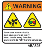
Figure 1. Fan Warning Nameplate
