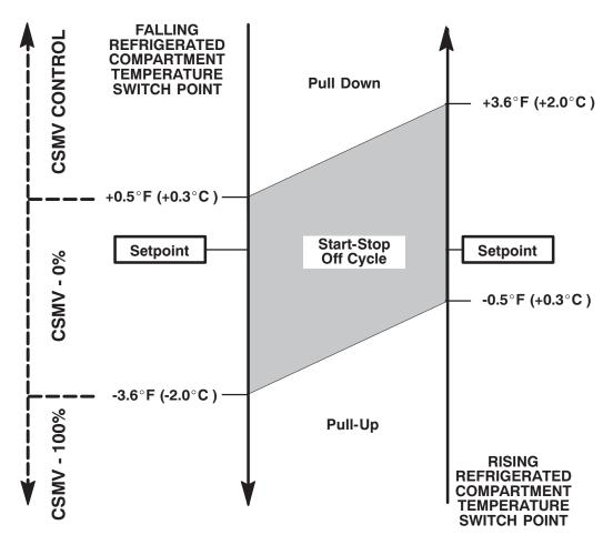
Switch Point = Controlling Temperature - Setpoint + results are above setpoint, - results are below setpoint
