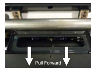
7. Remove the upper fan shroud bolts, and remove the shroud.
