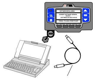
PC–USB Service Cable. Carrier Transicold Part #: 22–04253–01 = 20 foot/6.1 meter long)
