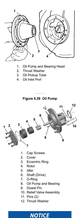
Ensure that thrust washer does not fall off dowel pins while installing oil pump.
