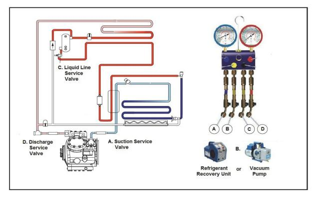
Figure 8.22 Four Port Manifold Gauge Option
