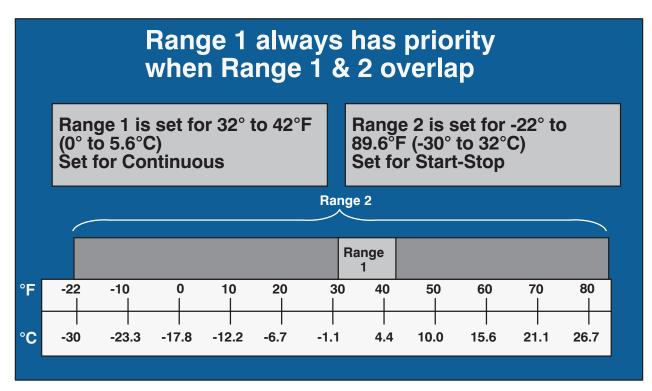
Typically, Range 1 and Range 2 are used to control different setpoint ranges when IntelliSet is not active. For units with IntelliSet, because each IntelliSet is generally programmed for a specific product, only Range Lock 1 is used to hold the unit in either the Start/Stop or Continuous Operation, and Range Lock 2 is left OFF.
